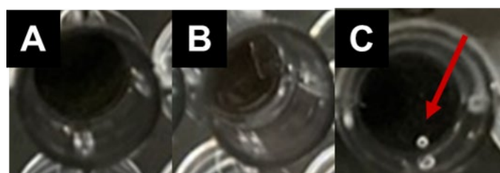
Figure 4.2. Catalase mimics of Au-based Nanozymes after 38 minutes. Control experiment, H 2 O 2 +Buffer (A). AuSeeds catalase mimics, H 2 O 2 +AuSeeds+Buffer; [Au] = 27 \mu M (B). LN/Au catalase mimics, H 2 O 2 +LN/Au; [Au] = 27 \mu M; [LiNbO 3 ] = 182 \mu M (C). For all the samples, the measurements were performed in the presence of H 2 O 2 (29.7 mM) at pH 4 (acetate buffer) and 37°C. All the concentrations are in the reaction well.
