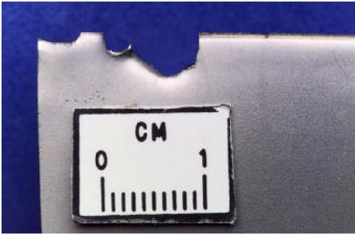
Figure 28 Blade damage due to surge (source: NASA)
