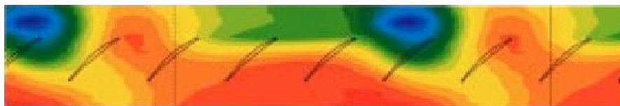
Figure 24 Pressure distribution over the rotor – visualization of the SLSD, (Inoue et al. , 2001, [41])
