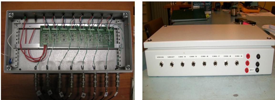
Figure 41 Pictures of the conditioners used for the unsteady pressure measurements (surface mount technology)
