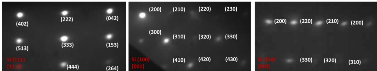
Figure 31. RHEED patterns obtained after the NW growth on: a) Si(111) along [112] azimuth, b) Si(100) along [001] azimuth and c) Si(110) along [001] azimuth. Ga pre-deposition: F_{Ga} = 0.5 ML/s, 2s at 400 °C; NW growth: F_{Ga} = 0.75 ML/s, 10 min at 570 °C, R_{V/III} = 10 .
