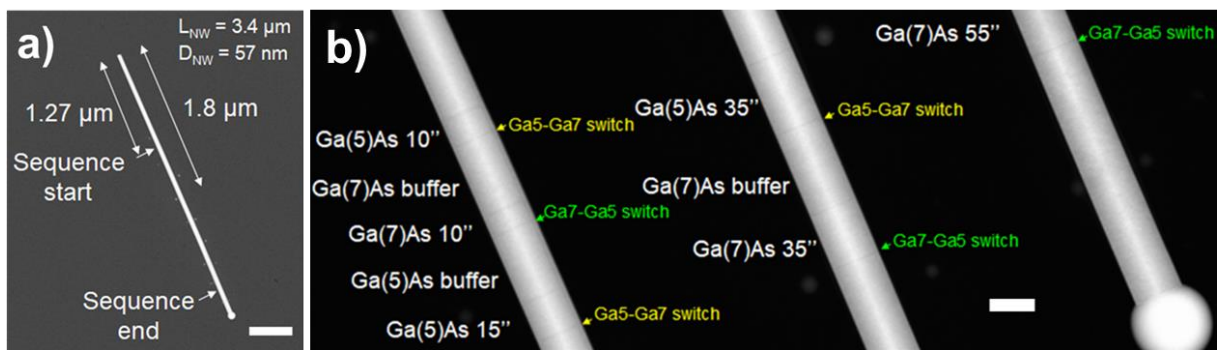
Figure 3.34. (a) TEM image of a GaAs NW showing the position of the sequence with alternated segments of Ga(5)As and Ga(7)As. (b) HR-TEM image of some Ga(5)As and Ga(7)As segments: the \text{Al}_{0.5}\text{Ga}_{0.5}\text{As} markers delimiting each segment can be observed. The moments of the Ga flux switches are also indicated. The white scale bars correspond to (a) 500 and (b) 50 nm, respectively.
