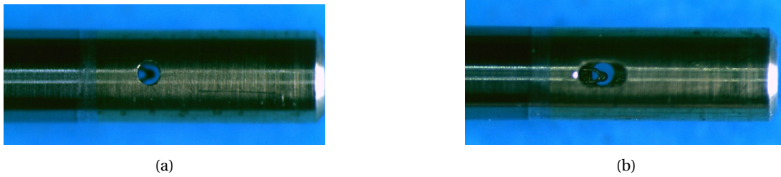
Figure 3.22: Ventilated Temperature probe for cavity flow investigation - (a) Front View - (b) Back view.
