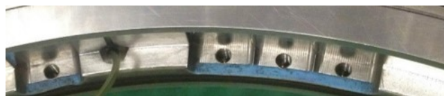
Figure 3.13: Holes for inserts in the stator platform - Instrumentation routing cable between two sensor sectors.
