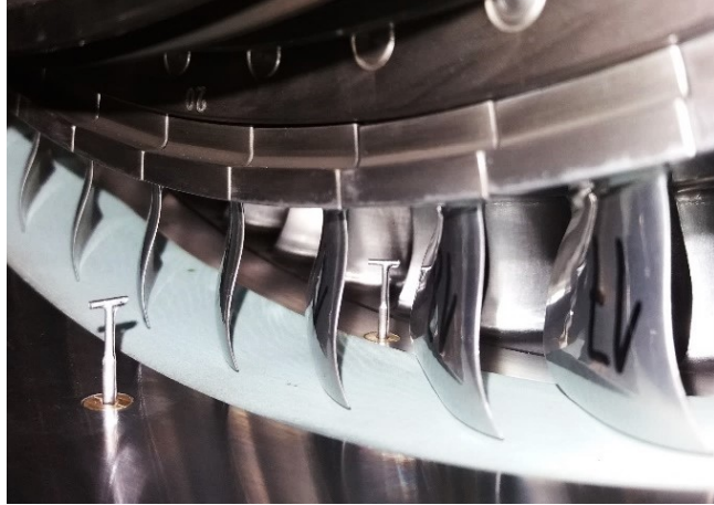
Figure 3.8: Miniaturized total temperature probes in Plane 1 and Plane 2.
