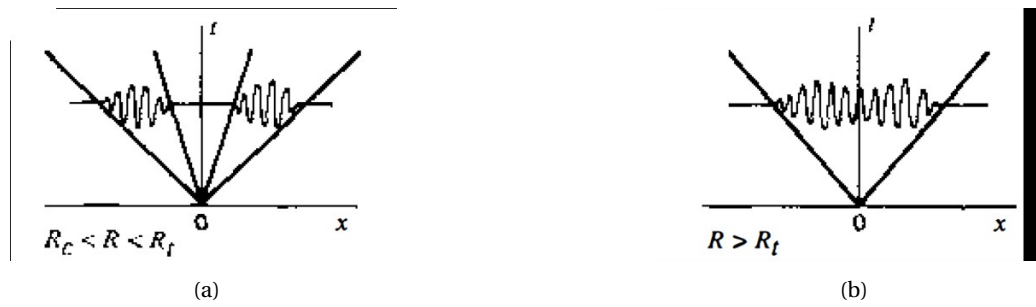
Figure 2.8: Impulse response to contra propagating travelling waves in (x: space, t: time) plane of parallel flows - (a) Convectively unstable - (b) Absolutely unstable - Huerre and Monkewitz (1990).
