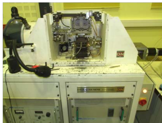
Figure 43: (a) Diagram and (b) photograph of the specific fretting apparatus.
